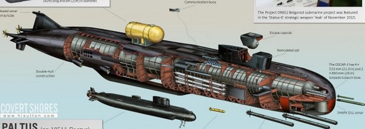
Labels in diagram: Towed sonar array tube, Communication buoy, Escape capsule, Remodeled sail, Double-hull construction, SHARK GILL sonar, The OSCAR-II has 4 x 533 mm (21.0in) and 2 x 650 mm (26 in) torpedo tubes in bow.
